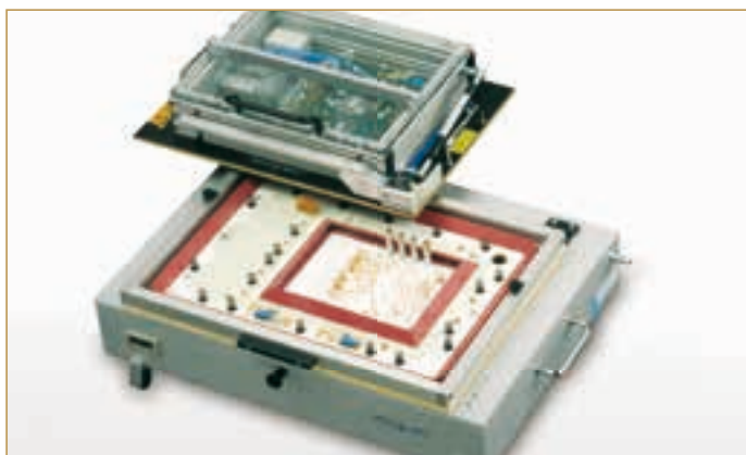
Dual-stage Test fixture with Vacuum-free Zone
